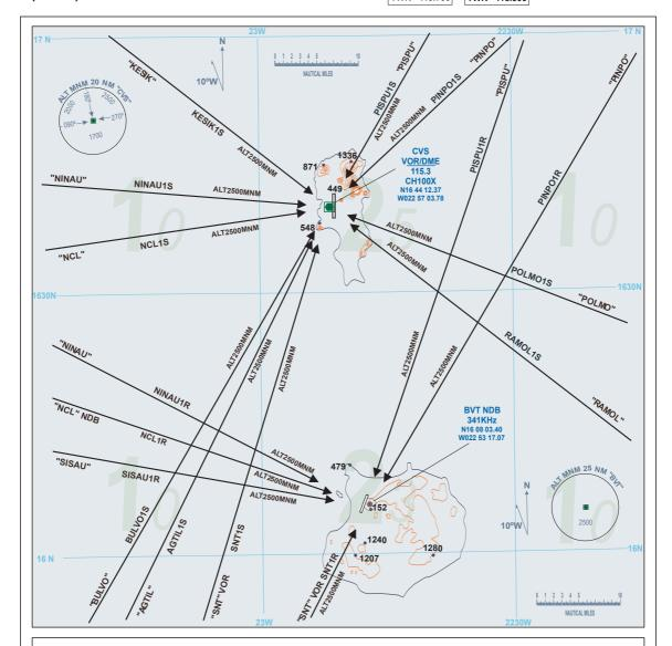
**Note**: Minimum safe altitudes (MSA) are indicated for each leg. Except in case of emergency or loss of communications altitudes to maintain are those assigned by ATC. These must respect the indicated MSAs.
