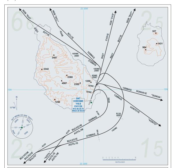
AGTIL1E: Climb on runway heading until passing 2500ft and 8DME/SNT. Turn right to join arc 10DME/SNT. Cross RDL130SNT at 6000ft or above. After crossing radial RDL180SNT follow track 270MAG to join RDL230SNT direct AGTIL.
